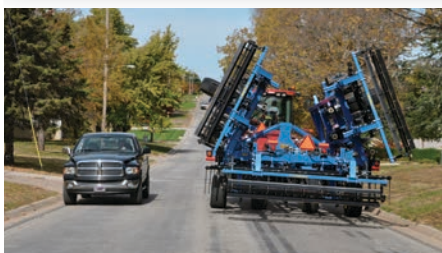
The 2430 – 11 and 13 Shank Model folds to an narrow 16' 0" width for transport.
